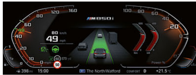
THE AUTOMATIC SPEED LIMIT ASSIST 1 * ADAPTS THE ACTIVE CRUISE CONTROL DYNAMICALLY TO UPCOMING SPEED LIMITS.
